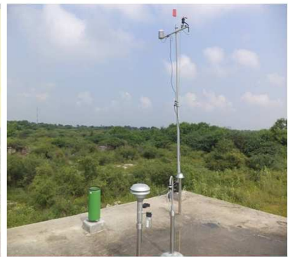
Wind direction, Speed & Rainfall Monitors
